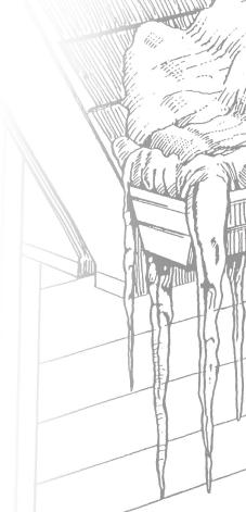
The result is water backing up under the roof shingles or behind fascia boards where it can soak through the roof decking or wall sheathing, causing damage to attics, ceilings and walls.
